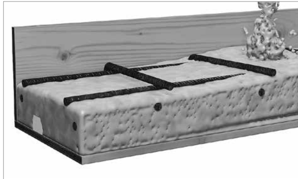
5. Concrete in the profile.
